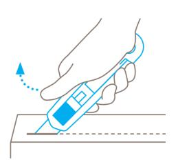
Always remove your **thumb from the slider** to For best results, cut plastic strapping band ensure automatic blade retraction.
