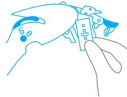
You can now lift up the blade cover to either **rotate or change** the blade.
